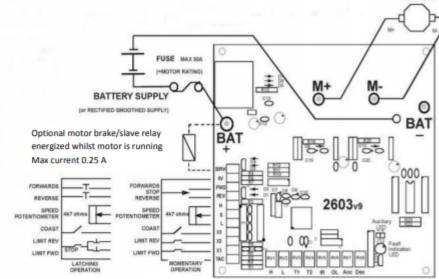
When the supply is on, the green LED should glow continuously. Selection of forward or reverse will permit the motor to run dependant on speed.
