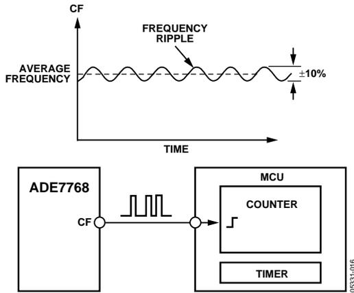
Figure 27. Interfacing the ADE7768 to an MCU
