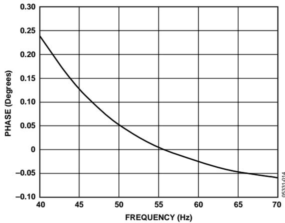
Figure 25. Phase Error Between Channels (40 Hz to 70 Hz)
