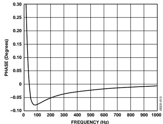
Figure 24. Phase Error Between Channels (0 Hz to 1 kHz)
