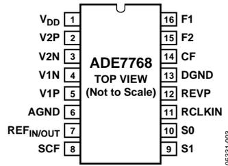
Figure 3. Pin Configuration
