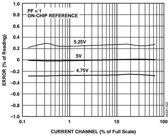
Figure 10. PSR with On-Chip Reference, PF = 1
