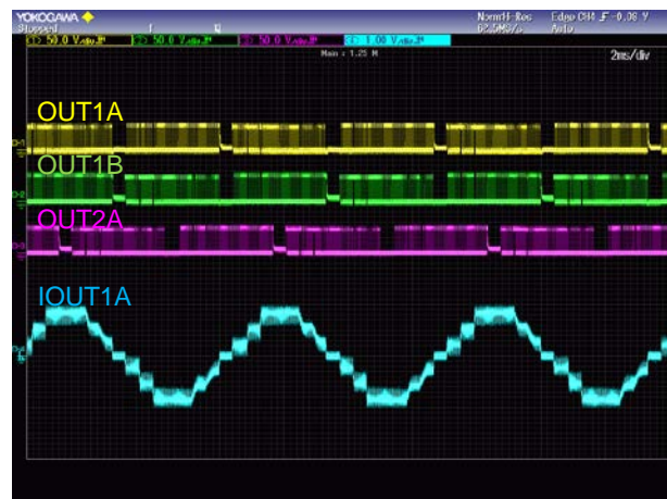
Figure 17. QUARTER STEP 駆動波形 ( CLK : 2400Hz )
