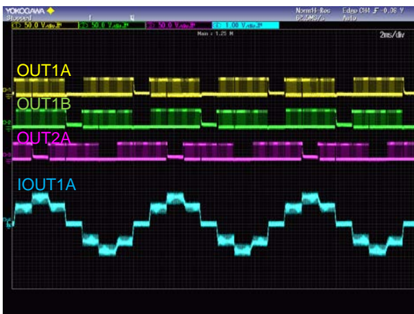
Figure 16. HALF STEP B 駆動波形 ( CLK : 1200Hz )
