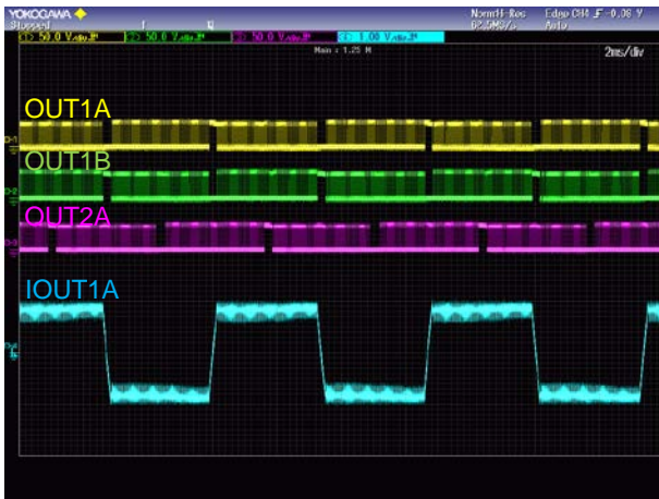
Figure 14. FULL STEP 駆動波形 ( CLK : 600 Hz )
