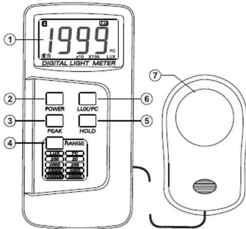
1. LCD Display: 3 ½ digits with a maximum reading of 1999.
