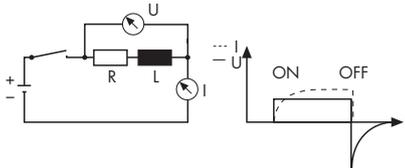
**Switching Relay Coils.**
