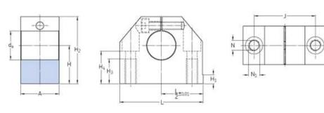
Design versions LSHS = Shaft blocks with ISO series 1 LBBR bearings LSNS = Shaft blocks with ISO series 3 LBC/LBH bearings
