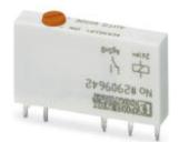
Plug-in miniature power relay, with multi-layer gold contact, 1 changeover contact, manual operation, 24 V DC input voltage
