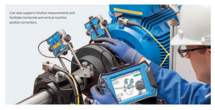
The advanced laser shaft alignment system with enhanced measuring and reporting capabilities
