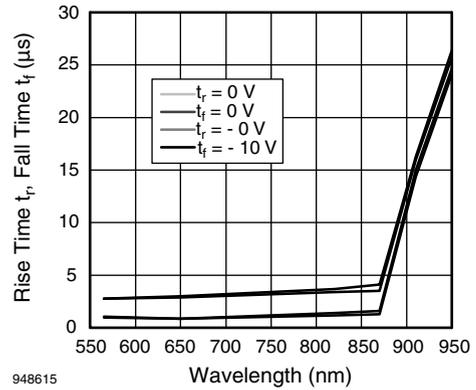
Fig. 25 - Switching Times vs. Wavelength for Photodiode BPW20RF
