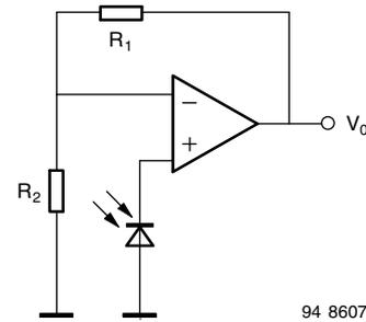
Fig. 17 - Photodiode in the Photovoltaic Mode Operating with a Voltage Amplifier
