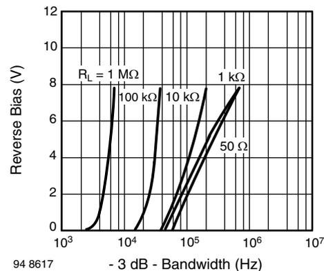
Fig. 27 - BPW41, TEMD5110X01, Bandwidth vs. Reverse Bias Voltage, Parameter: Load Resistance  $\lambda = 950$  nm
