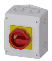
SENTRON, Switch disconnector 3LD, emergency switching-off switch, 3- pole, lu: 63 A, operating power / at AC-23 A 400 V: 22 kW, Molded plastic encapsulation for metric cable gland, 1 NC, 1 NO, rotary operating mechanism, red/yellow
