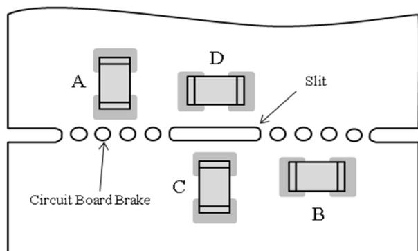
Stress strength according to the mounting position:
