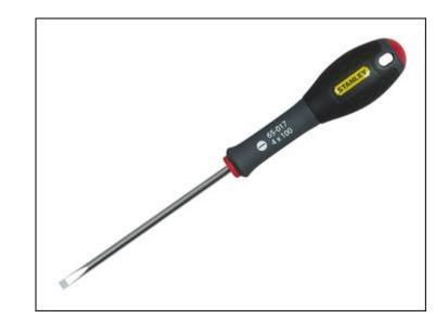
The FatMax Parallel tip screwdrivers have a chrome vanadium steel bar which allows high torque and reduces the risk of tip breakage, and the handle is moulded directly to shaft for a virtually unbreakable bond which gives long life and durability.
