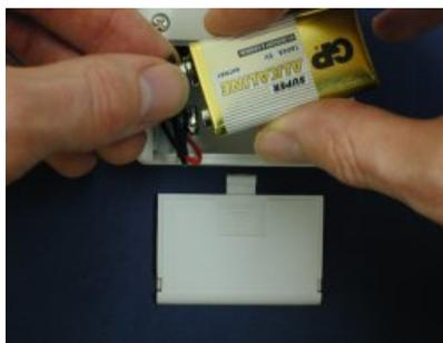
The pictures above show the removal of the battery. The reverse procedure should be used to replace the battery.
