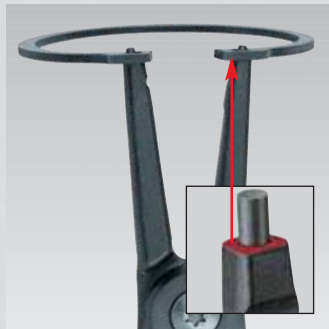
Circlips are held securely: large contact faces and the position of the tips make it difficult for the circlip to bounce off
