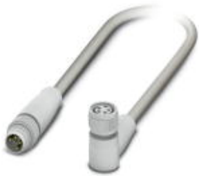
Sensor/Actuator cable, 4-position, PP-EPDM halogen-free, Gray RAL 7035, Plug straight M8, on Socket angled M8, Cable length: 0.6 m, Hygienic design, with plastic knurl
