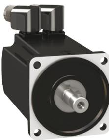
servo motor MH3 100 3,3Nm,no key,single 16 lines,brake,IP65/IP67,4kRPM
