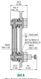
(Max. fluid level of the hydraulic reservoir between the banjo bolts)
