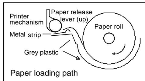
Check that the paper still advances properly, and tear off any excess by pulling the paper sharply towards you across the serrated edges. In the event of a jam or other paper loading problem, raise the paper release lever (as shown in the diagram) and carefully withdraw the paper, checking that no scraps have been left in the mechanism. Discard any damaged paper from the end of the roll, lower the paper release lever, and try again.
