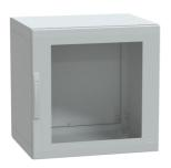
Floor standing polyester enclosure, PanelSeT PLA, glazed door, completely sealed, 750x750x620mm, IP65, IK08
