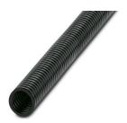
Protective hose, material: PA 6, UV-resistant: yes, flexible, degree of protection: IP68, color: black, flammability rating in acc. with UL 94: HB, inside diameter: 16.5 mm, Total length: 50 m
