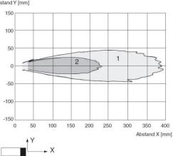
Curve1:flat surface 100mm×100mm Curve2:round bar,Φ25mm
