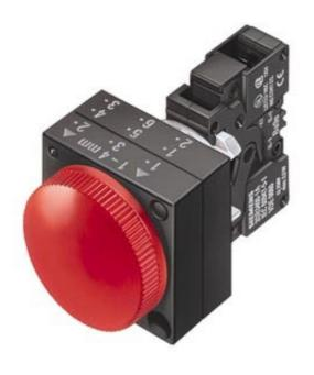
22MM PLASTIC ROUND COMPLETE UNIT COMBINATION: INDICATOR LIGHT WITH SMOOTH LENSE ILLUMINATED WITH INTEGRATED LED 24V AC/DC SPRING-LOADED TERMINAL WITH HOLDER RED
