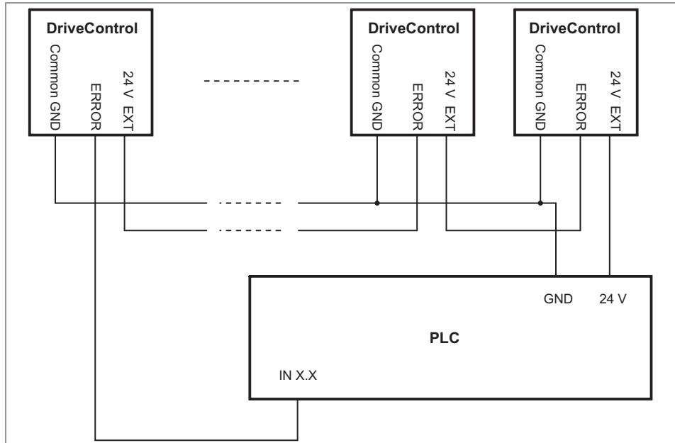
When operating voltage is disconnected, the ERROR output switches to the error condition. This ensures correct display of faults when the error signal of several DriveControl has been linked and the operating voltage of a DriveControl is switched off or if a cable defect (e.g. loosened contact, cable rupture) occurs.
