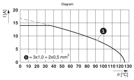
I = current strength, θ = ambient temperature, 3x 14 A + 2x 2 A constant
