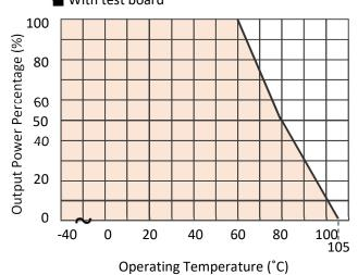
The derating curve was measured with nominal line. Mounted test board.
