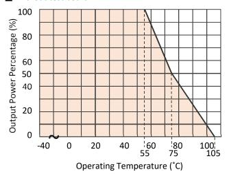
The derating curve was measured at nominal Vin in chamber with nature convection.
