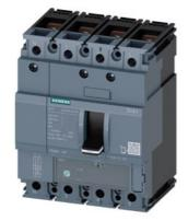
circuit breaker 3VA1 IEC frame 160 breaking capacity class S Icu=36kA @ 415V 4-pole, line protection TM220, ATFM, In=50A overload protection Ir=35A...50A short-circuit protection Ii=10 x In N conductor unprotected nut keeper kit
