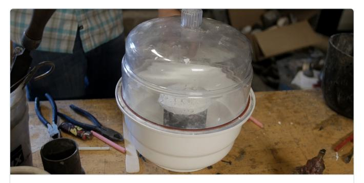
Degas the filled casting flask in the vacuum chamber again. Place filled casting flask on flat surface and allow to dry according to manufacturer's instructions. Remove the rubber sprue base and allow investment to dry for another two hours.
