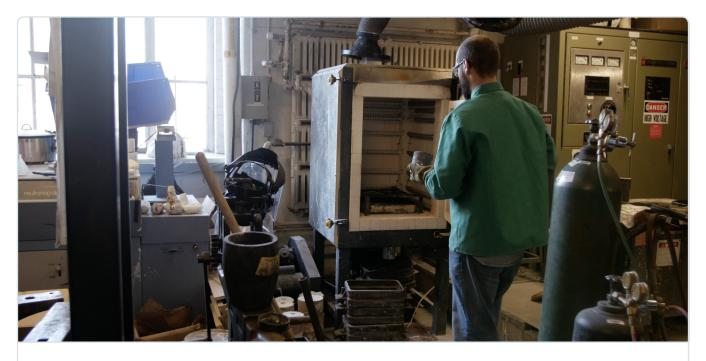
Place casting flask in a furnace and heat according to the burnout schedule provided on page 2. Remove the mold from the furnace. Cast as you normally would. Casting is an involved process. For best results, work with a casting specialist.
