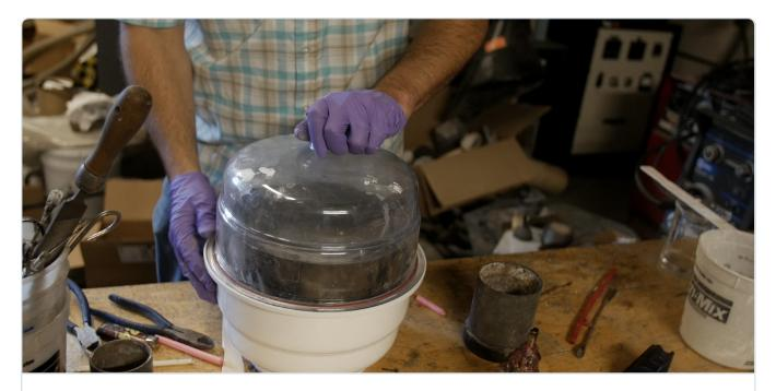
Degas the container with mixed investment in a vacuum chamber.
