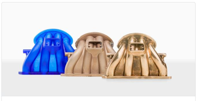
L – R: 3D printed manifold in Castable Resin, cast in brass, and after final polishing.
