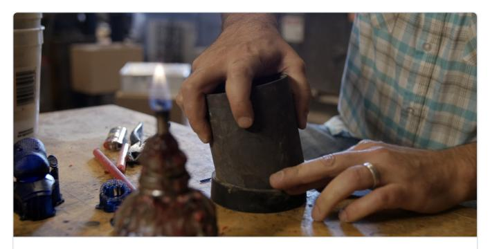
Attach a casting flask to the rubber sprue base.
