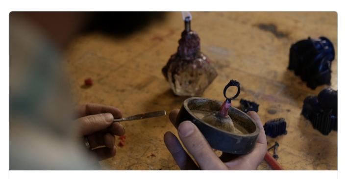
Attach the part to a rubber sprue base using softened wax. Make sure the wax is as smooth as possible.
