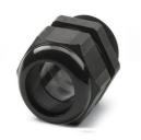
Cable gland, material for screw connection: PA, application: Standard, external cable diameter 30 mm ... 36 mm, shielding: no, connecting thread: M50 x 1.5, color: jet black RAL 9005
