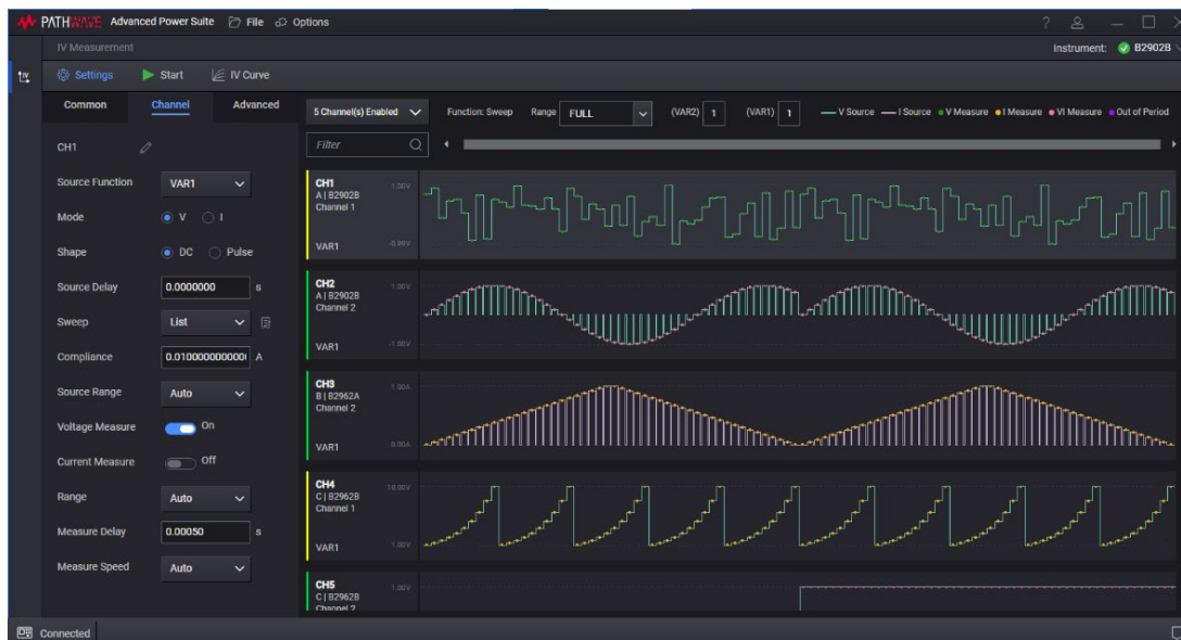
Figure 1. Previewing the settings of multiple SMU channels
