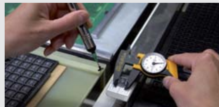
The dialMax ESD calliper can be used for measuring delicate electronic components.
