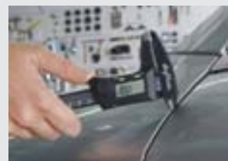
The measuring jaw of the fibre-glass reinforced calliper enables scratch-free measurement of even very delicate, shiny surfaces.
