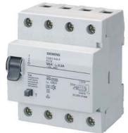
Residual current operated circuit breaker, 4-pole, type A, selective, In: 125 A, 300 mA, Un AC: 400 V  $\,$
