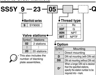
Type 23 manifold of Series SY9000 is concurrently used for the internal and external pilot.
