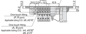
$\textbf{SS5Y3-45S1} \square \textbf{D-} \underline{\textbf{Stations}} \, \textbf{B-} \underset{\textbf{C6},\, N7}{\textbf{C4},\, N3} \, \textbf{-Q} \, \, (\text{for SI unit types C, Q, R1, R2 and V})$
