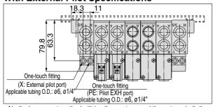
\* Air discharge port on the built-in silencer type and the external pilot's extracting position are in the B side (both sides).
