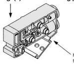
Hook the DIN rail here and press down in the direction of the arrow until a click sound is heard.
