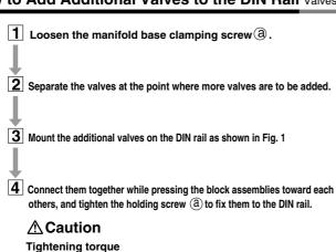
(While lightly holding the blocks after fixing an end block on one side, tighten the other end block for better sealing after no gap between valves is confirmed.)
