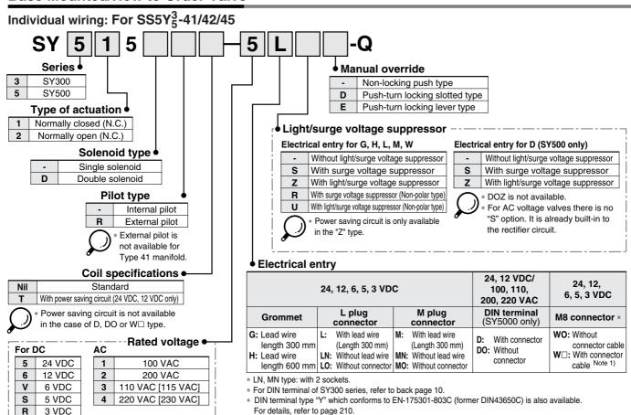
For connector cable of M8 connector, refer to back page 12.
