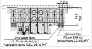
\* Air discharge port on the built-in silencer type and the external pilot's extracting position are in the B side (both sides).
