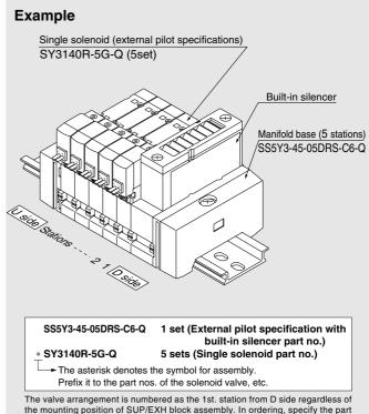
The valve arrangement is numbered as the 1st. station from D side regardless of the mounting position of SUP/EXH block assembly. In ordering, specify the part nos. in the order from the 1st. station on D side. Besides, when the arrangement will be complicated, fill out the manifold specification sheet to instruct us. For manifolds with SUP/EXH block assembly at each end of the manifold, external
