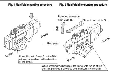
⚠ Caution When clamping screw @ of the end block is not sufficiently tightened during reassembly, air leakage may result. Before supplying air, check that there are no gaps between valves and that the end block is firmly secured to the DIN rain in order to ensure air supply without leakage.
