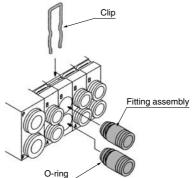
Type 45 manifold permits change in the A and B port sizes by changing the manifold block fitting assembly.
