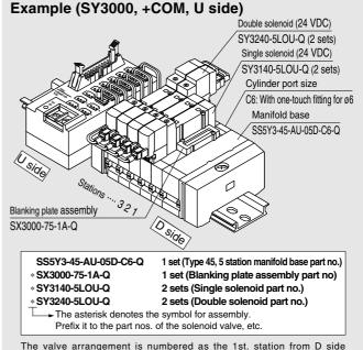
The valve arrangement is numbered as the 1st. station from D side regardless of the mounting position of connector box. In ordering, specify the part nos. in the order from the 1st. station on D side. Besides, when the arrangement will be complicated, fill out the manifold specification sheet to instruct us.
