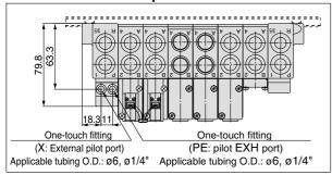
\* Air discharge port on the built-in silencer type and the external pilot's extracting position are in the U side.
