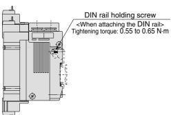
$\ast$  When P, R port outlets are indicated on the U side, the P, R ports on the opposite side are plugged.
