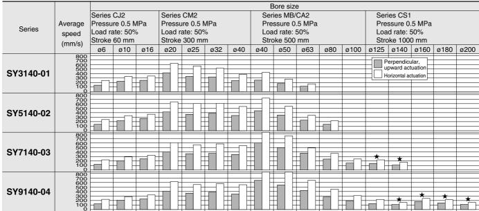
Cylinder is in extending. Speed controller is meter-out, which is directly connected with cylinder and its needle is fully opened.
