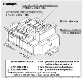
The valve arrangement is numbered as the 1st. station from D side regardless of the mounting position of SUP/EXH block assembly. In ordering, specify the part nos. in the order from the 1st. station on D side. Besides, when the arrangement will
