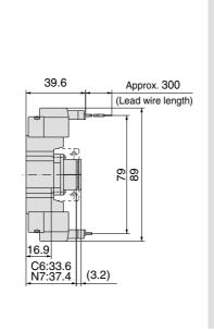
M plug connector (M): SY3220- $\square$ M $\square$ - $\overset{C4}{C6}$ ,  $\overset{N3}{N7}$ (- $\overset{1}{F_2}$ ) -Q
