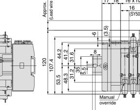
L dimension: Formulae for L1, L4  $L3 = 12.5 \times n1 + 16 \times n2 + 70$  $M= (\frac{L3}{12.5} + 1) Omit decimals$ L1 = 12.5 x M + 23 L2 = L1 - 10.5L4 = (L1 - L3)/2
