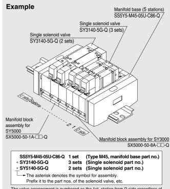
The valve arrangement is numbered as the 1st. station from D side regardless of the mounting position of SUP/EXH block assembly. In ordering, specify the part nos. in the order from the 1st. station on D side. Besides, when the arrangement will be complicated, fill out the manifold specification sheet to instruct us.
