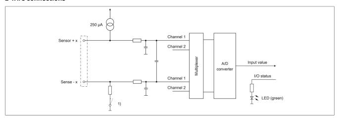
1) Switch is closed for 2-wire connections.
