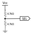
**NOTE:** Recommended to use  $2 \times 4.7$ -k $\Omega$  resistors (Vcc-GND).
