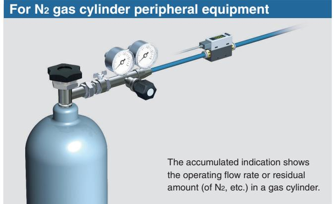
The accumulated indication shows the operating flow rate or residual amount (of N<sub>2</sub>, etc.) in a gas cylinder.
