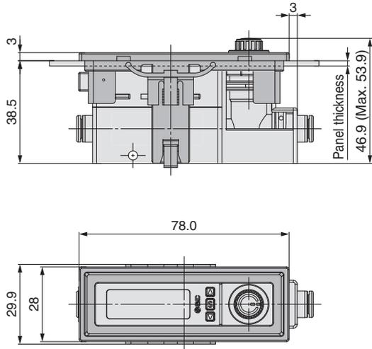
With bracket/With flow adjustment valve
