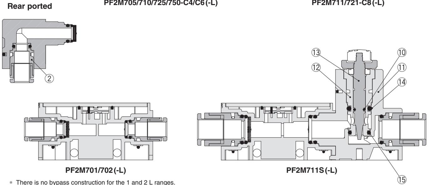
\* There is no bypass construction for the 1 and 2 L ranges.
