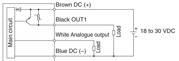
Max. load current: 80 mA, Internal voltage drop: 1.5 V or less
