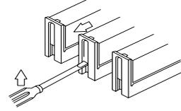
Notes: 1. Exercise care when removing relays. If greater than necessary force is applied at the socket hooks, deformation may alter the dimensions so that the hook will no longer catch, and other damage may also occur.
