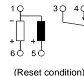
Since this is a polarized relay, the connection to the coil should be done according to the above schematic.
