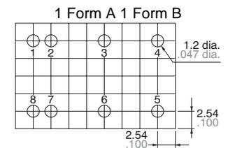
The above shows 2 coil latching type. No.2 and 7 terminal are eliminated on single side stable type.
