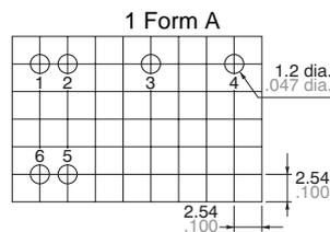
The above shows 2 coil latching type. No.2 and 5 terminal are eliminated on single side stable type.
