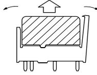
4. In case there is not enough space to grasp relay with fingers, use screwdrivers in the way shown below.
