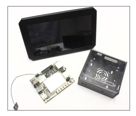
1. Start by inserting the ribbon cable on the back of the screen through the slot in the base of the PCB housing.
