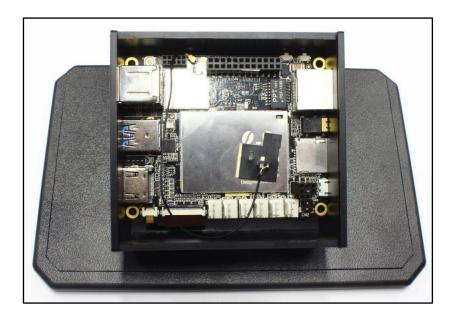
4. Once the PCB is in place ensure that the components on the sides line up with their cut-outs and then slide the clear cover into place.
