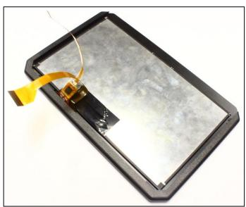
2. Insert the ribbon cable through the slot on the back panel and begin to slide the panel back on. - You will need to pull the cable through as you go.
