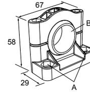
**Hole center spacing:** A=ø 50.8
