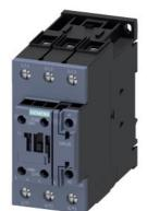
power contactor, AC-3e/AC-3, 41 A, 18.5 kW / 400 V, 3-pole, 20-33 V AC/DC, 50/60 Hz, with integrated varistor, auxiliary contacts: 1 NO + 1 NC, screw terminal
