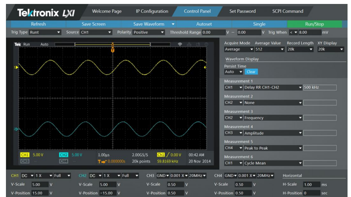
LXI control screen and waveform display enable remote control over Ethernet
