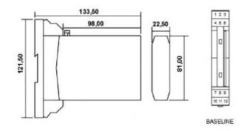
Dimensions: width: 22,5 mm - Height: 81 mm - Depth: 98 mm
