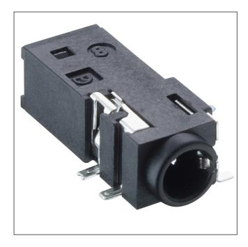
Jack chassis socket according to JEITA RC-5325A, 3.5 mm, 4 poles/stereo, with break contact, angular version, for printed circuit boards, surface mount technology (SMT)
