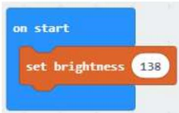
Result: the brightness of the whole LEDs is 138
