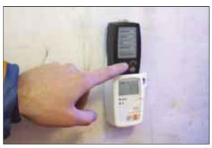
The pocket-size testo 580 - data collector transfers data from loggers on-site for PC download
