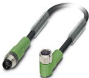
Sensor/Actuator cable, 3-position, PVC, black RAL 9005, Plug straight M8, on Socket angled M8, Cable length: 1.5 m
