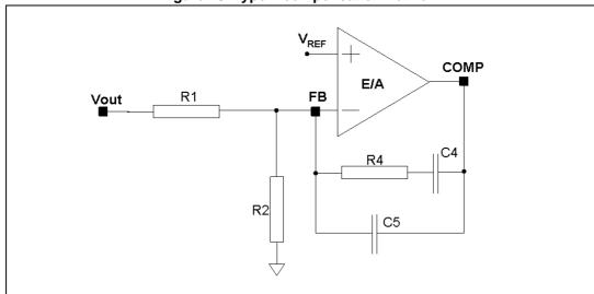
Figure 13. Type II compensation network
