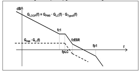
Figure 14. Open-loop gain: module Bode diagram
