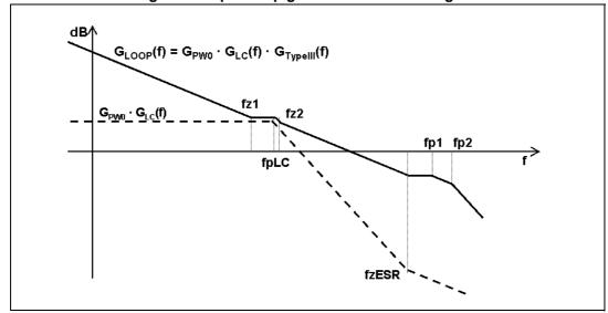
Figure 11. Open-loop gain: module Bode diagram
