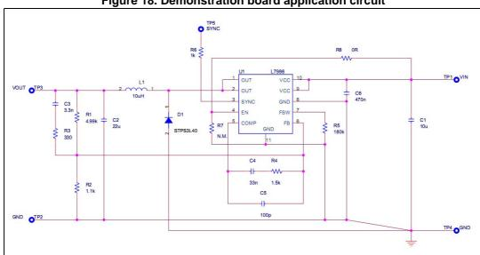
Figure 18. Demonstration board application circuit
