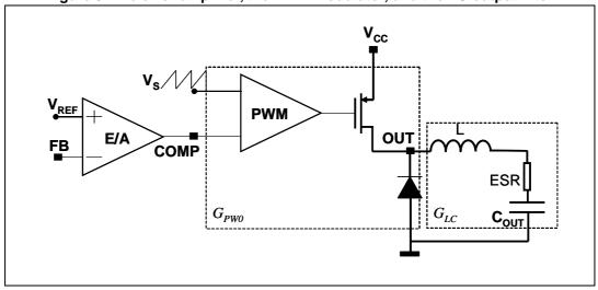
The transfer function on the LC filter is given by:
