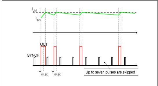
Figure 8. Overcurrent protection
