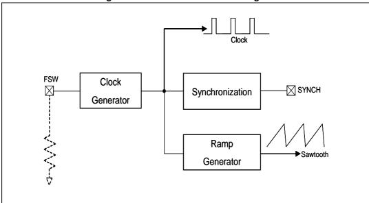
Figure 4. Oscillator circuit block diagram
