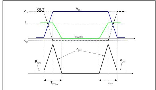
Figure 16. Switching losses
