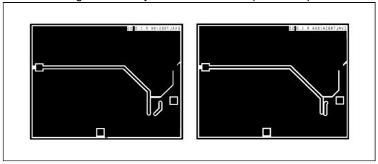
Figure 21. PCB layout: L7986 and L7986A (front side)
