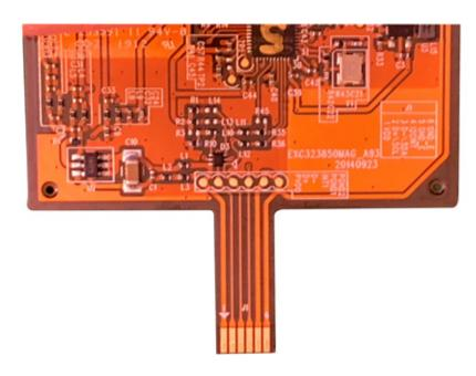
Remove any packing foam and tape to release the Touch control board from the back of the display. Place the display face up and line up the small USB connector PCB.
