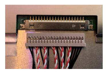
Connect the backlight connector from the driver card to the back of the LCD
