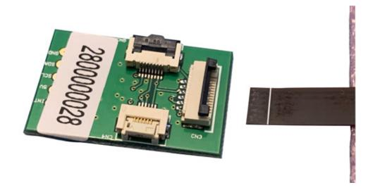
Note the orientation of the FFC and the PCB, it must be connected the correct way round or damage may occur. Push the FFC tail into the connector far enough so that the dark strengthening section is all the way in, and close the flap.
