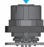
5. Mate the Connector Waterproof Cover (XS2Z-22, sold separately) or the Partner Connector Plug (XS5H-T42□-□M0-K, sold separately) and press the O-ring to the O-ring position after mounting.
