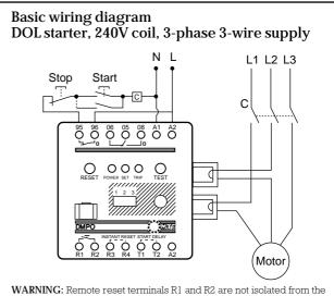
WARNING: Remote reset terminals R1 and R2 are not isolated from the supply. The remote reset contact, if used, and its associated cabling, must withstand supply voltage. The contact loading is 2mA at 20Vdc. Output terminals 05, 06, 08 - 95, 96 are for control circuit use in accordance with IEC 947 Parts 4 and 5. They should not be used for isolation purposes.
