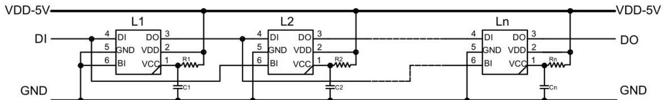
Remarks: Rx is the IC's protective resistor, power spike and reverse connection of the battery power terminal, will be protected, its range of 100R~300R. VCC & VDD are connected together without use of protective resistors. C1 is external filter capacitor, its value of 100NF. The LED also works without the external filter capacitor because it has filter capacitor built-inside.
