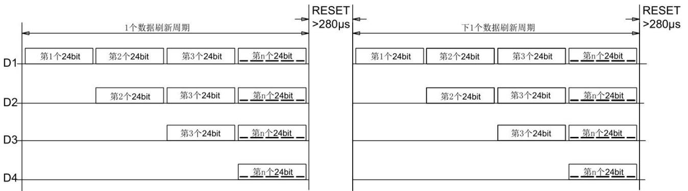
Note: D1 is the data from MCU, and D2, D3, D4 are from Cascade Circuits.
